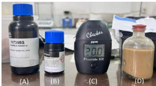
Figure 3. Fluoride analysis setup using the Portable Fluoridimeter (Hanna Checker Fluoride High Range). (A) HI739BS Fluoride HR Reagent B, (B)
