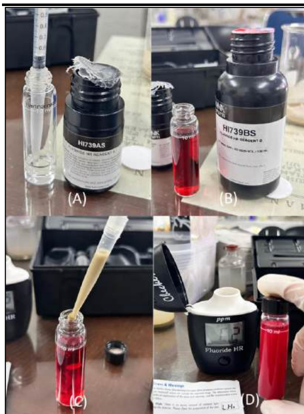
Figure 1. Step-by-step fluoride analysis procedure using Hanna Checker Fluoride HR. (A) Addition of 2 mL Reagent A (HI739AS) into a 10 mL cuvette. (B) Addition of Reagent B (HI739BS) until the cuvette reaches the 10 mL mark, resulting in a red-colored solution. (C) S. commersonnii was added to the reagent solution using syringe. (D) The cuvette containing the test mixture is inserted into the Hanna Checker Fluoride HR device for fluoride concentration measurement.
