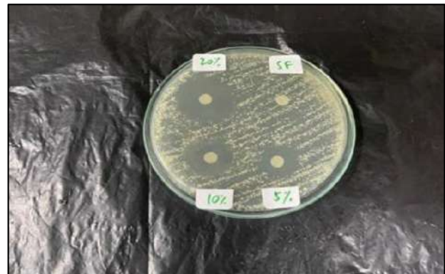
Figure 1. Diameter of inhibition zone formed from the addition of propolis to infant formula
