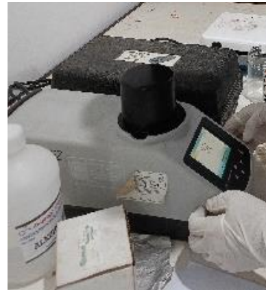
Figure 1. (Color measurement with ColorFlex EZ spectrophotometer)
